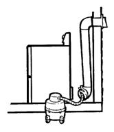
Inspect and clean the dryer exhaust ducting at least once a year to prevent clogging. A partially clogged exhaust can lengthen the drying time.
